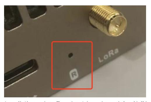
Answer: No, it's not reset button. The reset button is the power button on the front of the Heltec Indoor Hotspot. Press once to reset, long press than 4 seconds to shut down.
